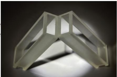
The SIM-6301-Q is a dual-window cuvette crafted from premium far-UV quartz glass (JGS1). Featuring  $\lambda/4$  surface flatness @632.8nm and strict dimensional tolerances of +0.0/-0.1mm, it delivers exceptional optical performance with matched pair transmission variance <0.5%.
