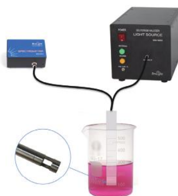
Immersion absorbance measurement
